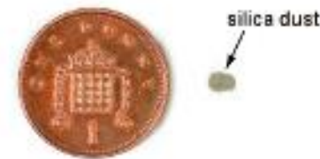
Figure 2 Your maximum daily silica exposure is tiny when compared to a penny.
